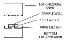
Lift the die set carefully and position it in the barrel of the Hand Press (please note, the top anvil may slide as it is not mechanically engaged with the bottom part of the assembly).
